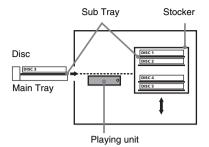
The disc changer consists of a playing unit and a stocker which transports the discs to the disc slot and the playing unit.
